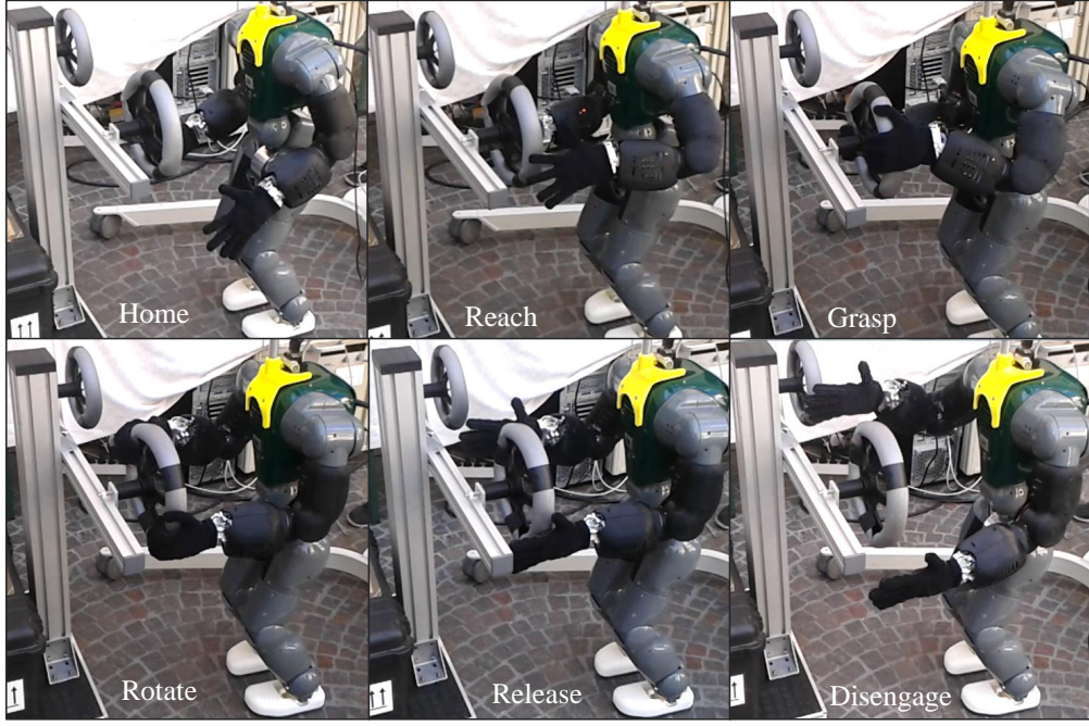
Fig. 6: Valve turning sequences, starting from the home posture: Reach, Grasp, Rotate, Release, Disengage. This sequence is repeated until the valve is open.
