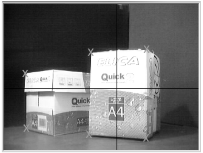
Fig. 9. Final servoed image. Note that image features correspond to the highlighted features in fig. 8, within the vision system noise.
