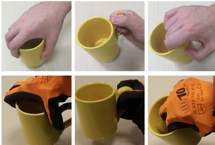
Fig. 15: A human hand grasping a cup with three different approaches (top panels) and the same grasps reproduced with the Pisa/IIT SoftHand (bottom panels).
