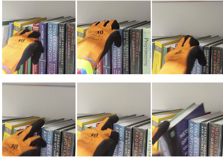
Fig. 17: A person with the arm-mounted SoftHand can seamlessly execute also difficult manipulation tasks which involve combined interactions between hand, object and environment.
