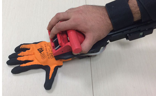
Fig. 16: The Pisa/IIT SoftHand mounted on an a human arm.
