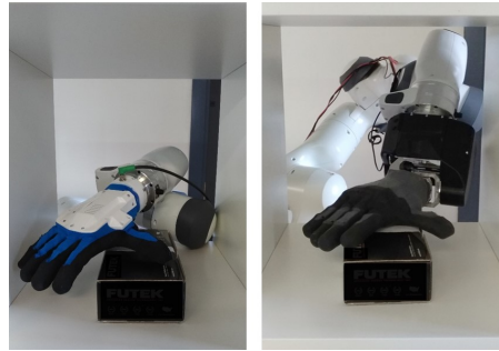
Fig. 1: Examples of robot grasping in a box with and without the Compact Soft Articulated Parallel Wrist (SWR).
