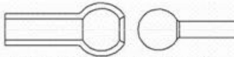
Figure 3: A ball and socket joint is a kind of annular snap fit.
