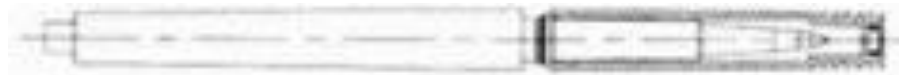
Figure 1: A pen sometimes utilizes an annular snap fit to retain the cap.
