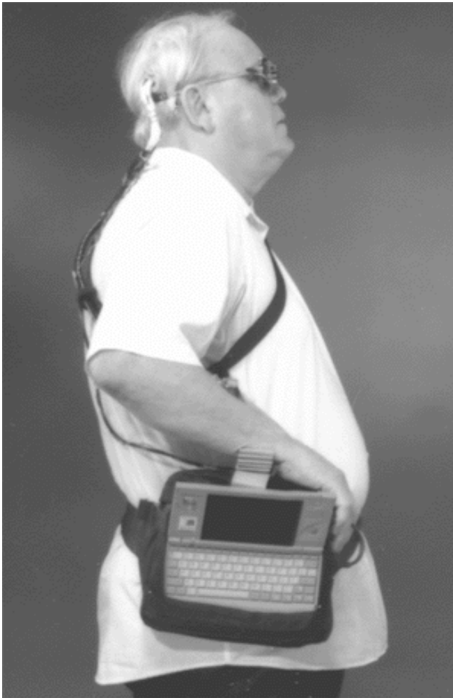
Figure 2. The complete artificial vision system showing the computer and electronics package on the belt with output cable to the electrodes on the brain.
