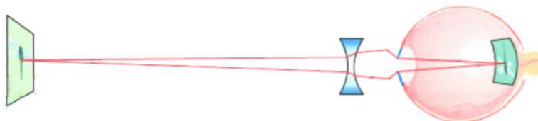
Figure 14.14 A corrective lens that diverges light rays before they enter the eye (i.e., a concave lens) will allow the myopic eye to focus the image of a distant object on the retina.
