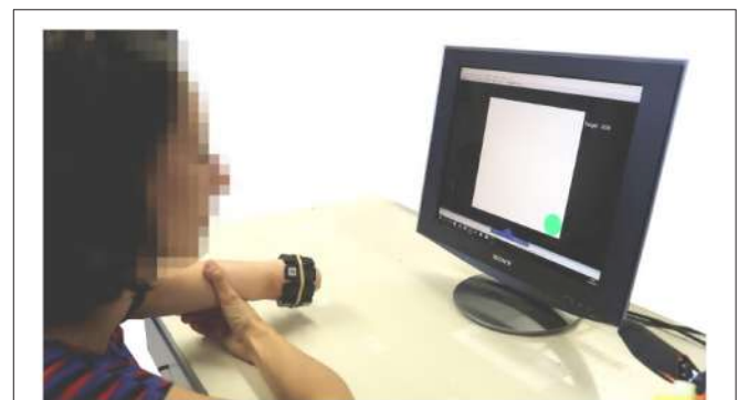
FIGURE 24 | The first Subject while performing the experiments in the virtual environment. The MYO Armband is placed on the setup. Both Map 3 and 5 are tested. The benchmark could not be tested because it was not possible to extract enough independent signals from the subject.
