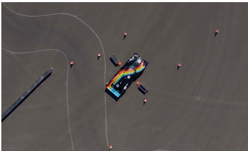
Figure 11. Top view of the Roborace DevBot 2.0 in Zala Zone Circuit. Narrow corridors (gates) were distributed along the track, the car is 2 meters wide, while the gates were 2.5 meters wide.
