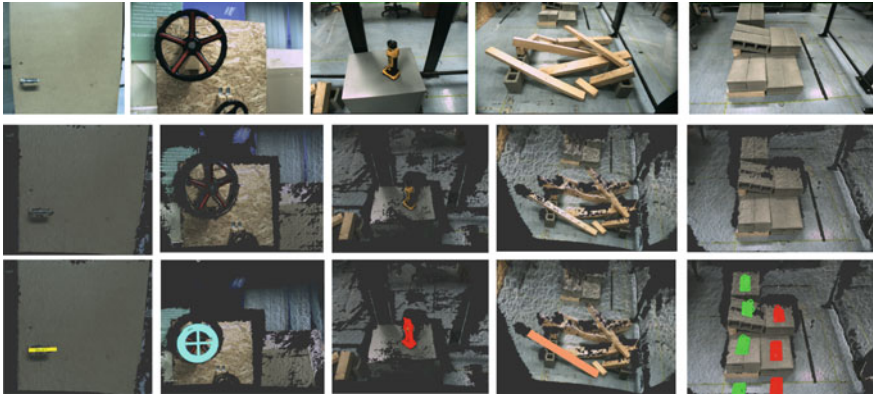
Fig. 38 Visual perception results for the door handle, the circular valve, the drill, the debris, and the rough terrain. The RGB image, the point cloud data, and the fitted model, appear in each row correspondingly
